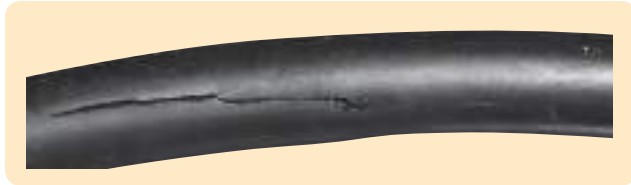
Figure 10-4: O-Ring Damaged by Explosive Decompression
