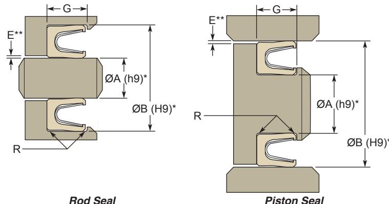
Each of these FlexiSeal profiles were designed to fit into the Metric glands on this page.
