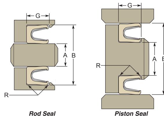
Each of these FlexiSeal profiles were designed to fit into either the Inch/Fractional glands on the following pages or the Metric glands on **Page 5-17**.
