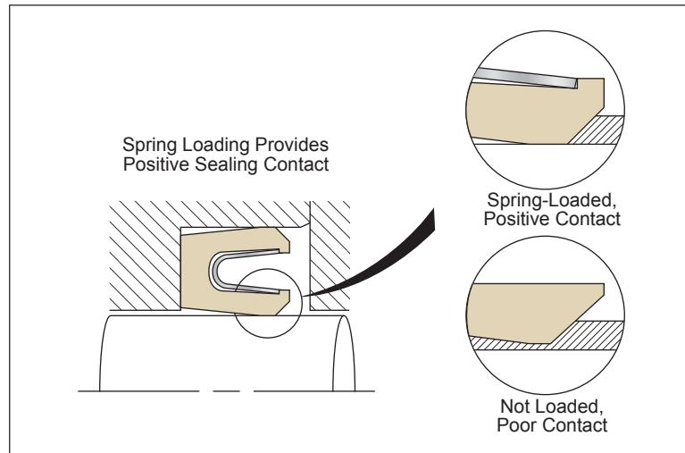
**Figure 2-14. Spring Loading**
