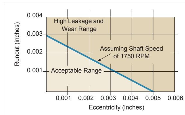
**Figure 2-25. FlexiLip and FlexiCase Eccentricity and Runout Limits**
