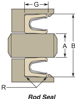
Each of these FlexiSeal profiles were designed to fit into the MIL-G-5514 rod glands on the following pages.
