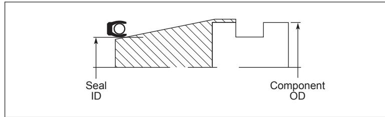
Figure 2-7. Place on Guide Ramp
