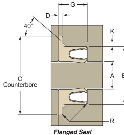
Each of these FlexiSeal profiles were designed to fit into either the Inch/Fractional glands on the following pages or the Metric glands on **Page 7-26**.
