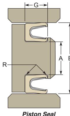
Each of these FlexiSeal profiles were designed to fit into the MIL-G-5514 piston glands on the following pages.
