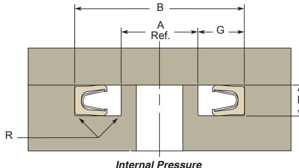
Each of these FlexiSeal profiles were designed to fit into either the Inch/Fractional internal pressure face seal glands on the following pages or the Metric glands on **Page 6-20**.
