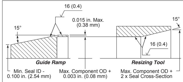
Figure 2-6. Stretching Guide Ramp and Resizing Tool
