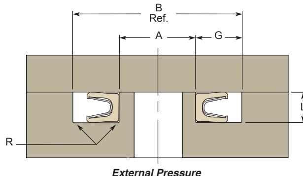
Each of these FlexiSeal profiles were designed to fit into either the Inch/Fractional external pressure face seal glands on the following pages or the Metric glands on **Page 6-20**.
