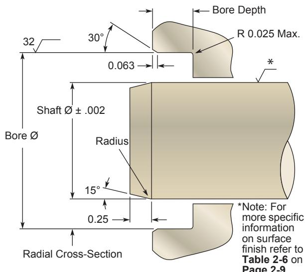
**Step 6** — Find minimum seal width from **Pages 9-8** to **9-9** and input into part number. Minimum seal width is always the most economical, but you can choose any width between the minimum recommended seal width and the actual bore depth. In this case you could choose any width between 0.200" and 0.500".
