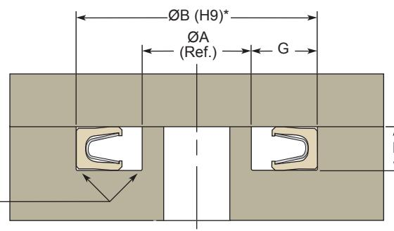
Each of these FlexiSeal profiles were designed to fit into the metric glands on this page.
