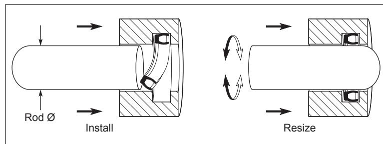
**Figure 2-10. Rod Seal Installation in Solid Gland**
