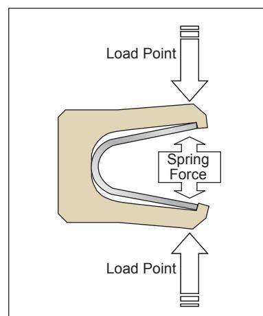
**Figure 2-16. Installed State**
